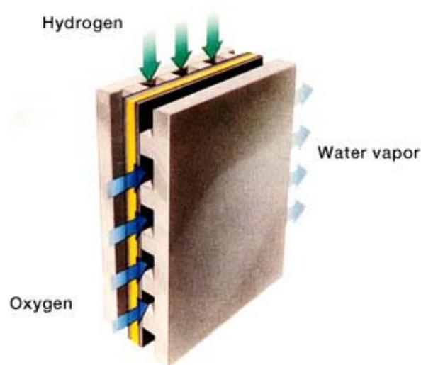
• Fig 4-2: Illustration of a layer of the fuel cell stack, how the gases pass through and water being produce. (HydroGen 1)
