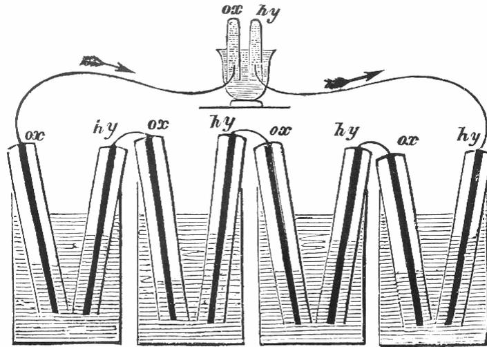
• Fig 2-1: Four Cells of Grove's  $H_2/O_2$  Battery to drive the electrolysis cell (Using  $H_2$  and  $O_2$  to electrolysis water) (Liebhafsky and Cairns, 20)
